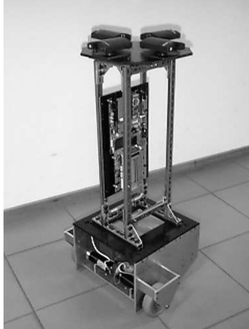
Figure 4.6: The inside core of the second version of the RoboGuard base. It includes a mobile PC-board and four color-cameras allowing full 360 degrees surveillance.
