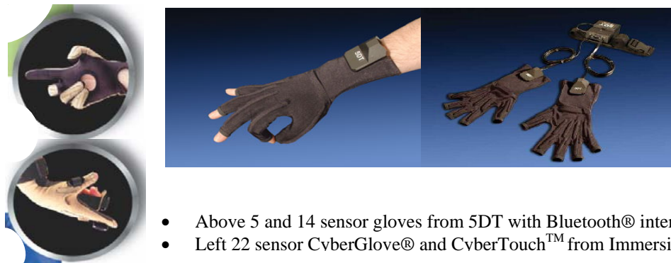
Fig. 2 “intelligent” virtual reality interaction gloves from Immersion and 5DT
